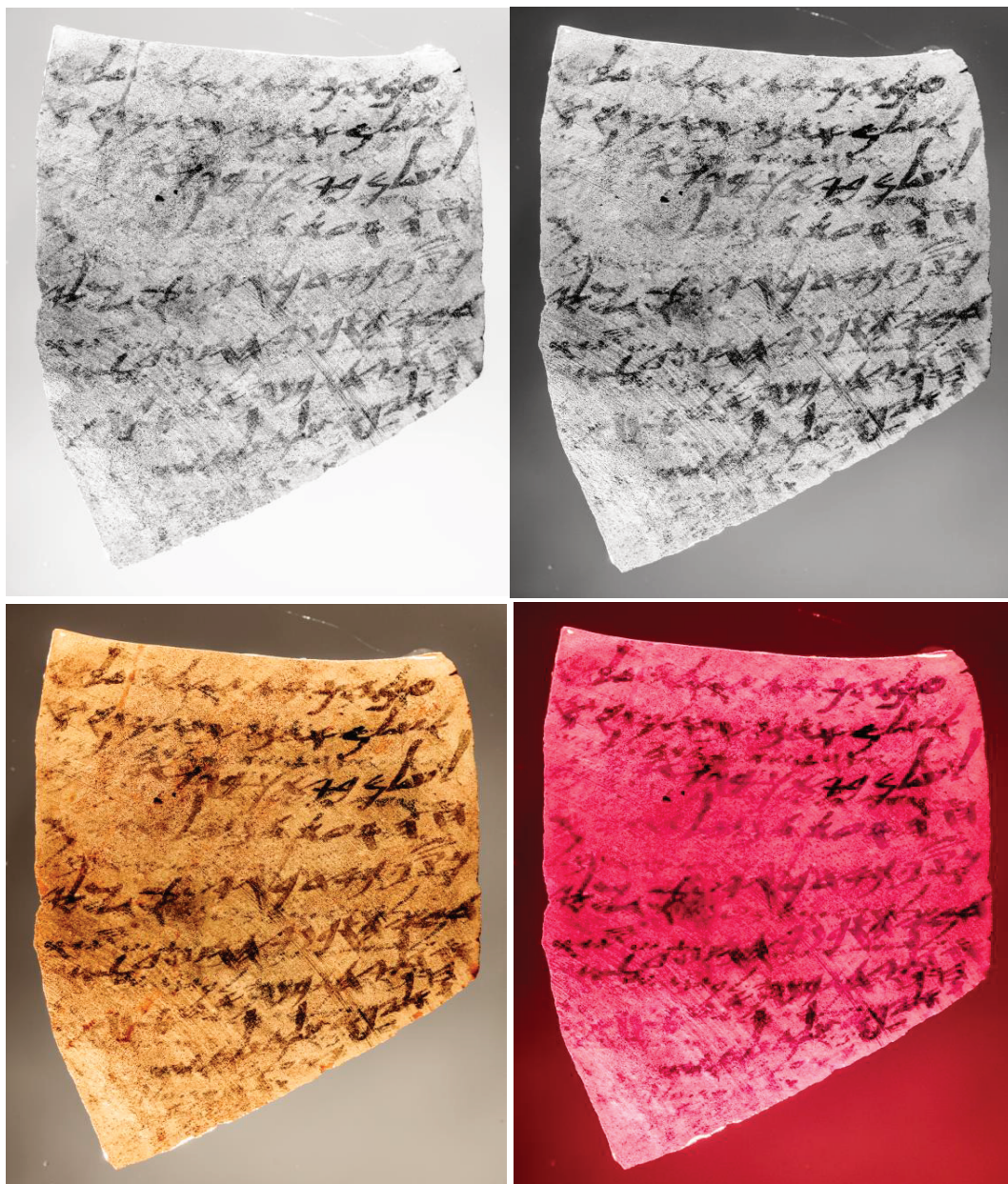
Figure 1. Multispectral imaging of JH433 A (convex side) after digital enhancement. From left to right and from top to bottom: (a) 470 nm; (b) 590 nm; (c) visible spectrum; (d) full spectrum
